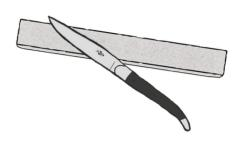
To maintain the optimum quality of the edge of your blade, we recommend a sharpening on natural stone. Moisten the stone for about ten minutes, then, keeping a sharpening angle of 20°, maintain a constant pressure by sliding the blade along the stone.
